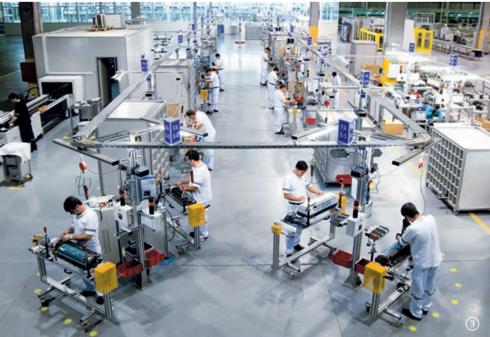
One-piece flow assembly in the Vaillant Group plant in Bozüyük, Turkey.
