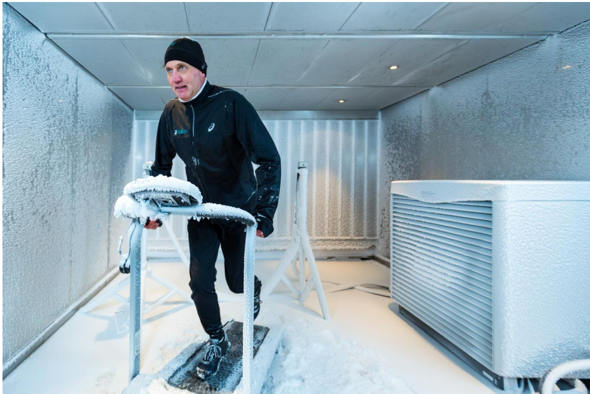
Image caption: Friedhelm Weidemann prepares for the extreme Antarctic temperatures in the climatic chamber at Remscheid-based heating and ventilation technology specialist Vaillant. The chamber is usually used to test heating appliances' cold-weather endurance.
