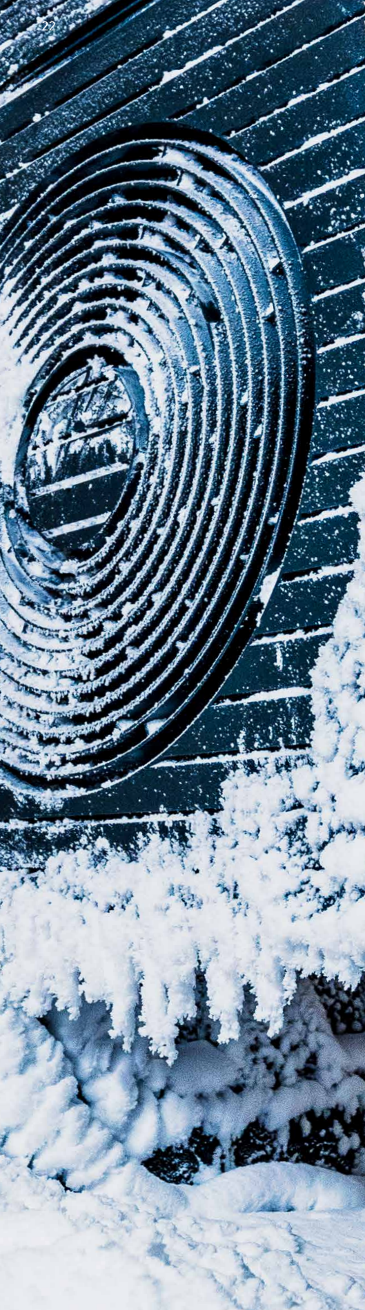
Heat pumps are exposed to extreme climatic conditions in the test chambers at the JOHANN VAILLANT TECHNOLOGY CENTER .
