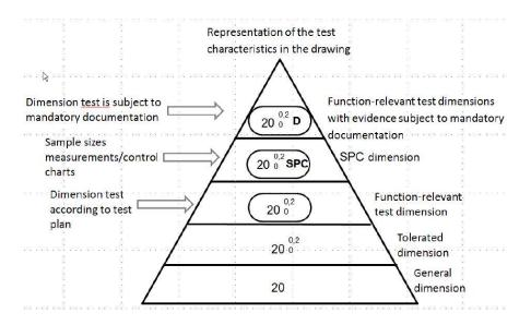
The VAILLANT GROUP drawings will define any significant characteristics, which are informed by the supplier's quality planning and/or risk analysis results (e.g., the production and/or process FMEA). These are highlighted in the VAILLANT GROUP specifications or drawings accordingly.
