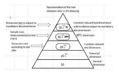
Any significant characteristics will be defined by the VAILLANT GROUP drawings, which are informed by the results of quality planning and/or risk analysis conducted by the supplier (e.g. the production and/or process FMEA). These are highlighted in the VAILLANT GROUP specifications or drawings, accordingly.
